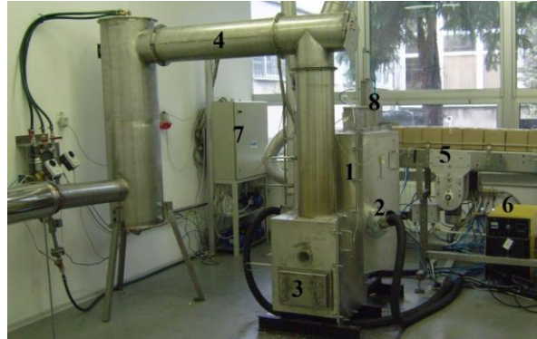
Figure 1. Overview of laboratory setup: 1) Plasma reactor, 2) Plasmatron, 3) Molten product collection, 4) Fumes Exhaust – chimney, 5) Waste package transporter, 6) Plasmatron power supply, 7) PLC – automation and data collection apparatus cabinet, 8) Automatic waste package feeder
